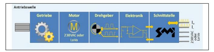
Figure 1: Basic construction of a SMI drive
